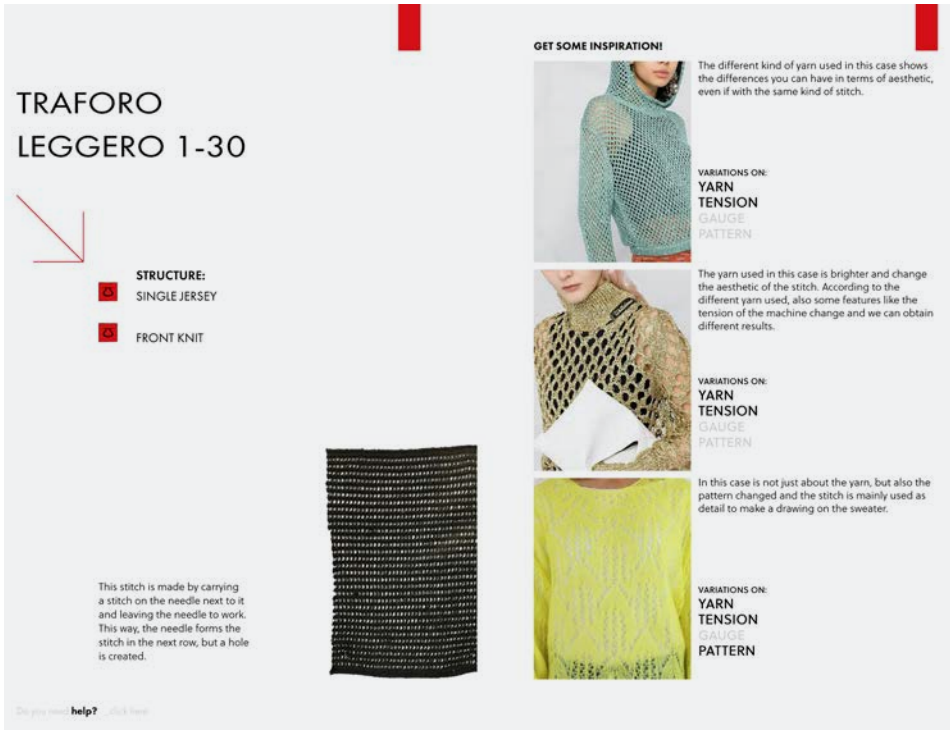
Figure 4. One of the 10 pilot technical sheets that contain: references to the consultation guidelines; color codes and symbols to identify the main features of the sample; detailed information on how the sample is made and could be replicated; possible variations with reference pictures that show what could happen when changing yarns, tension, machine gauge, pattern. Authors, 2022.
