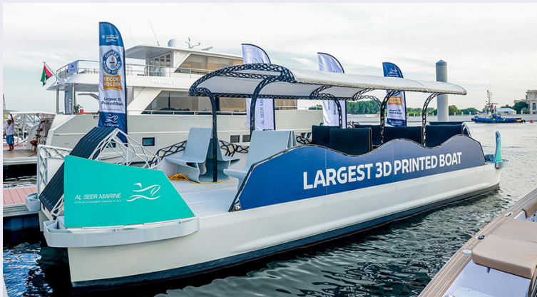
Figure 14. 3D printed electric water taxi by Al Seer Marine. Credits: Abu Dhabi Maritime.
