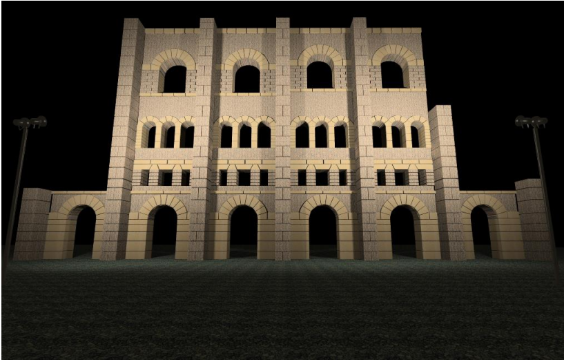
Figure 4.42 The luminaires were placed on two six-meter-high poles and further off-center to increase the shadow contrast of the vertical pillars in order to decrease the flattening of the façade. The tilt of the luminaires is decreased thus containing the upward scattered light flux.
