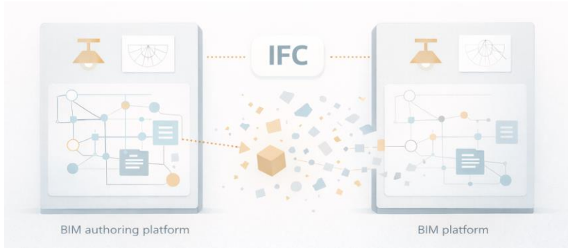
Figure 1.8 Interoperability in Open BIM workflows: during data exchange through IFC formats, semantic and parametric information—particularly for specialized objects such as lighting fixtures and photometric data—may be partially simplified, fragmented, or lost in translation between different platforms.
