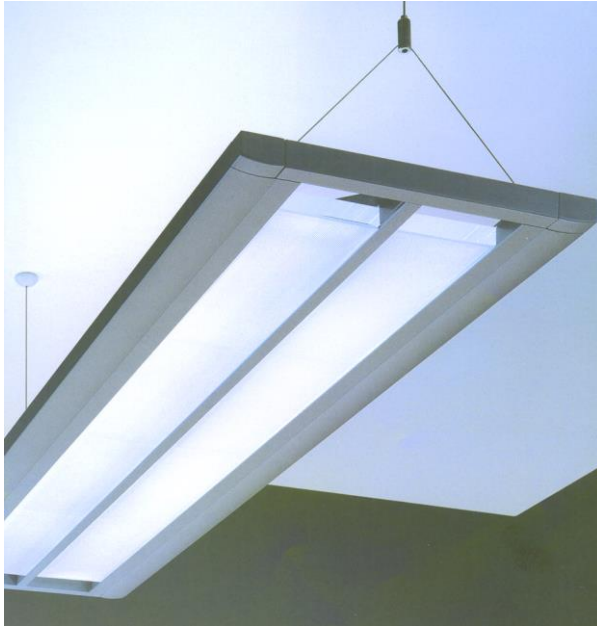
Figure 2.39 - Example of the use of RepTiles. The Aero luminaire designed by Sottsass Associati contains two linear fluorescent sources closed at the sides, the light is channelled through a BEF-type film. Courtesy Zumtobel Staff.
