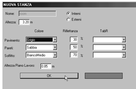
Figure 2.3 Example of the definition of reflection factors for the main surfaces of a room.
