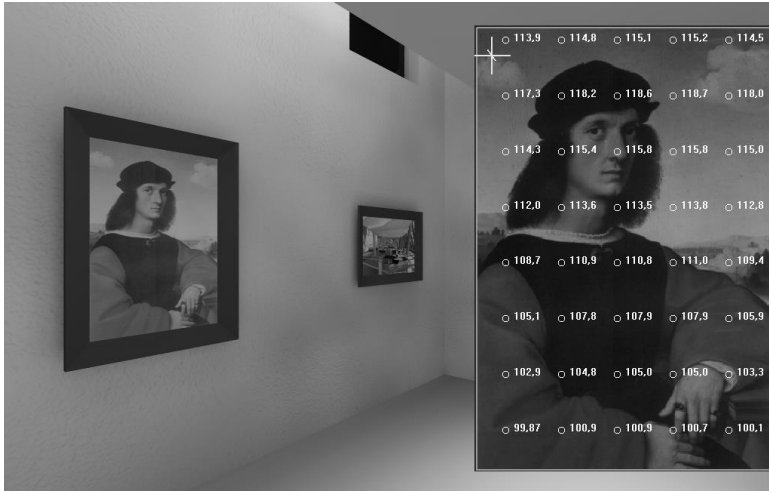
Figure 4.56 Illumination of a painting by indirect illumination with linear fluorescent lamps placed in the skylight recesses on the ceiling. Illuminance on the surface of the painting is visible on the right. The uniformity is very good, E_{\min} / E_{\text{med}} = 0.89 and E_{\max} / E_{\min} = 1.21 , with an average illuminance of 109 lux.
