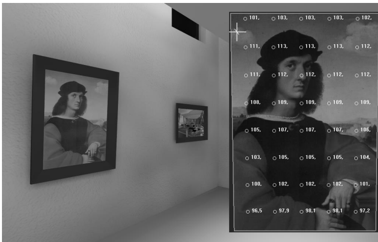
Figure 4.57 Compared with the previous figure, the painting has been tilted 4^\circ downward. Average illuminance decreased by 5 lux, while uniformity ratios deteriorated slightly: E_{\min} / E_{\text{med}} = 0.88 and E_{\max} / E_{\min} = 1.22 .
