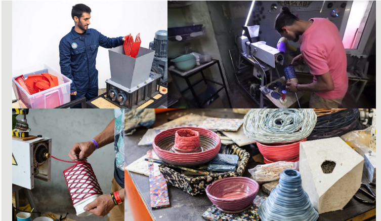
Fig. 3.33 Top-left: precious plastic machines (plastic shredding and fusion) at work; Top-right: extrusion and design of the new object in progress; Bottom-left: detail of a new object in production; Bottom-right: outputs of the precious plastic process 53
