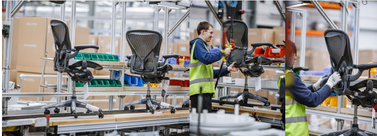
Fig. 3.4 Left: Aeron chair; Middle and right: Easily assembly and disassembly based on four screws and a single screwdriver 20
