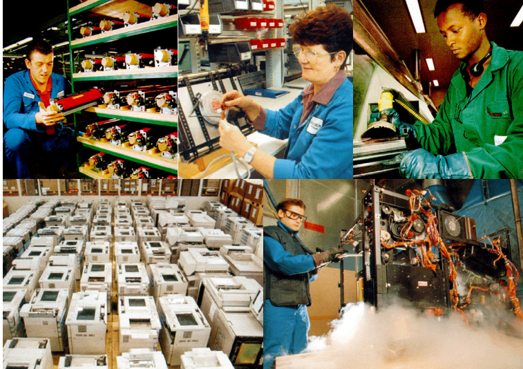
Fig. 3.32 Top: Xerox employees during test and maintenance operations on different components; Bottom-left: printers in the warehouse waiting for disassembly and check-up operations; Bottom- right: tests on functional printer core 52
