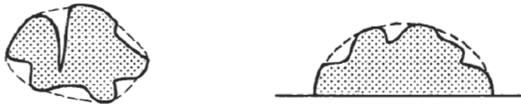
Figure 4: Irregularly Shaped Cracks
