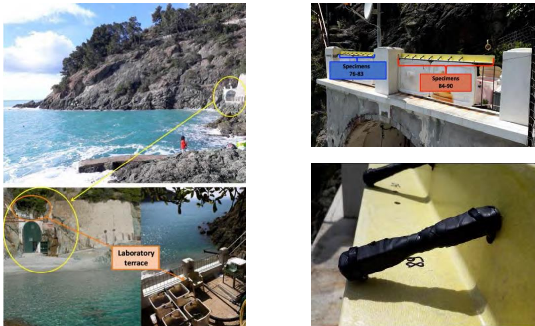
Figure 16: Exposure Rack on the Terrace of MARECO CNR-ICMATE Laboratory
