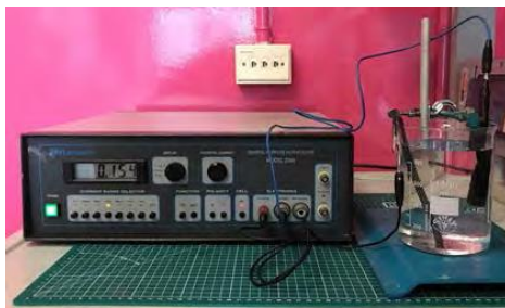
Figure 12: Setup of the Galvanostatic Test
