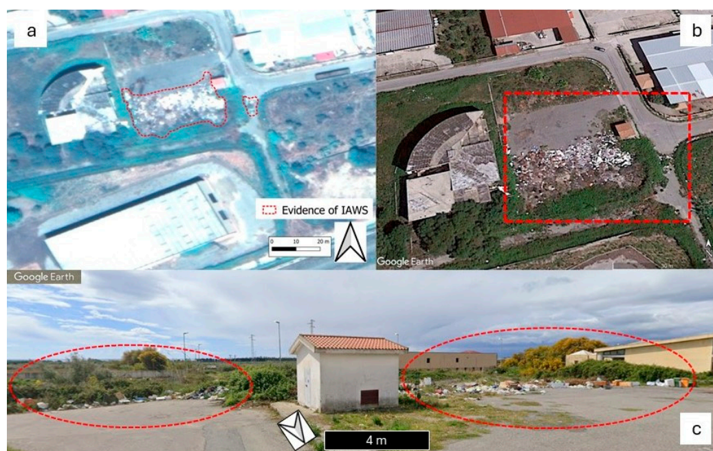
Figure 7. Identification of potential IAWSs in the municipality of Cropani through satellite and street-level pre-recognition analysis. The three images are described as follows: (a) Pansharpening results from WorldView-3 image (July 2021) for the study area; (b) image from Google Earth platform (May 2021); (c) image from Google Street View (April 2021).
