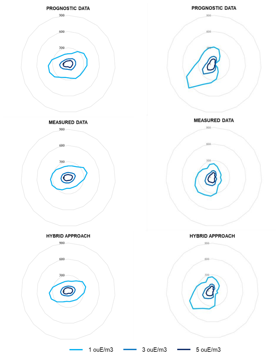
Figure 1. Odor impact maps for the European domain (left) and American island domain (right)
