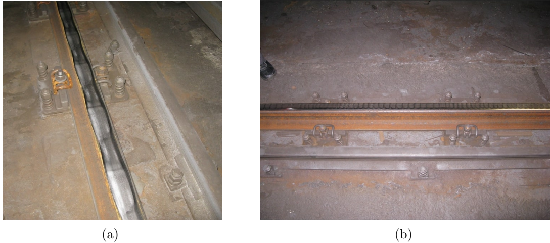
Figure 1.: Rail corrugation demonstrations on sections of rail from a metropolitan rail network.
