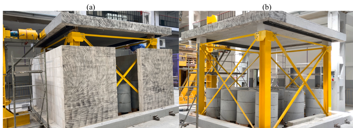
Fig. 2. Procedure for building models: (a) cutting off the walls from the slab, (b) demolishing the walls of a previously tested model with visible concrete weights designed to induce initial compressive stresses in the walls.
