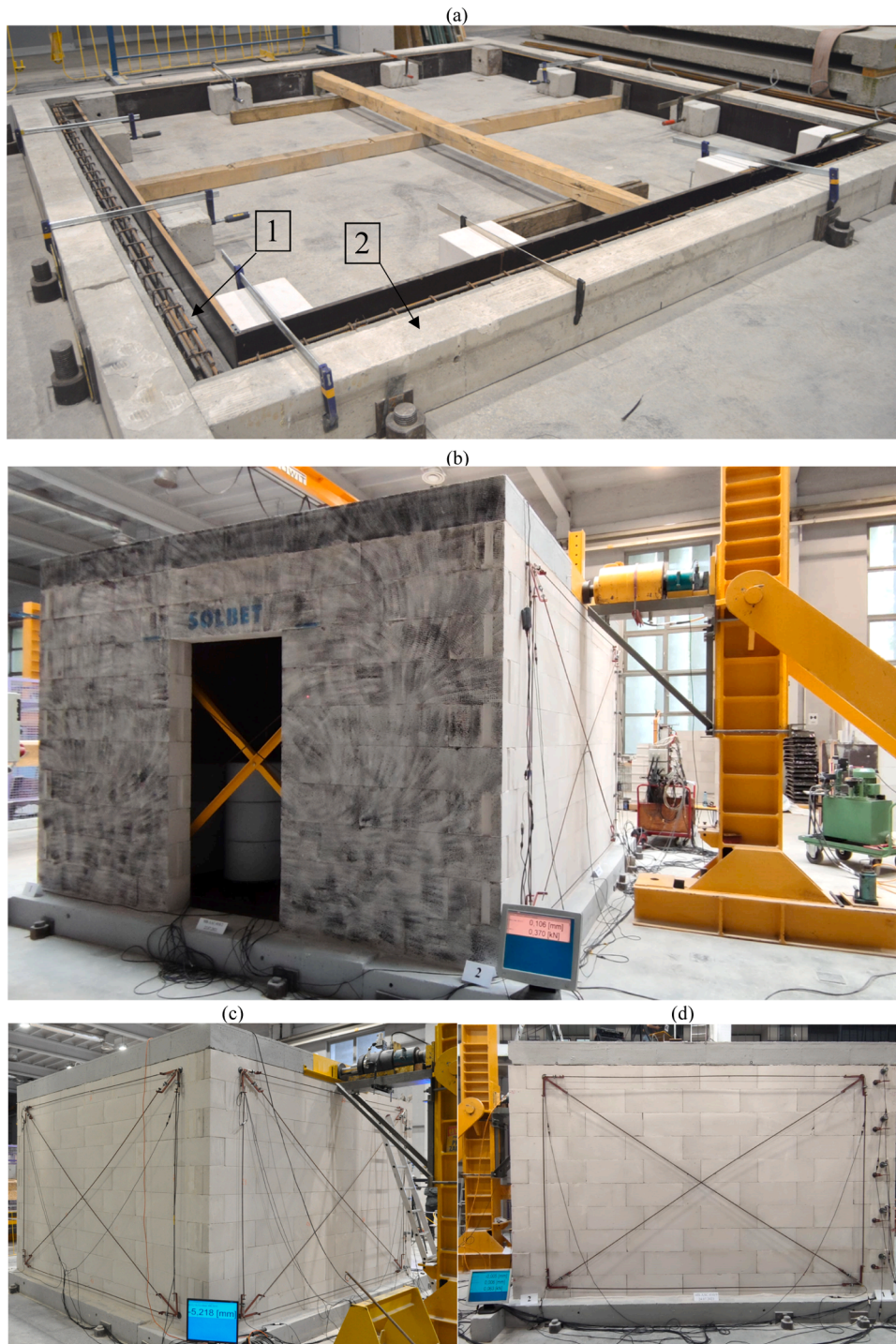
Fig. 3. Building models on the test site: (a) construction of the foundation for masonry walls, (b) model 2 with visible steel column and hydraulic actuator, (c) corner view of model 8, (d) stiffening wall view of model 9. 1 – reinforcement of foundation, 2 – extra concrete beams along the perimeter to guarantee the model remains fixed.
