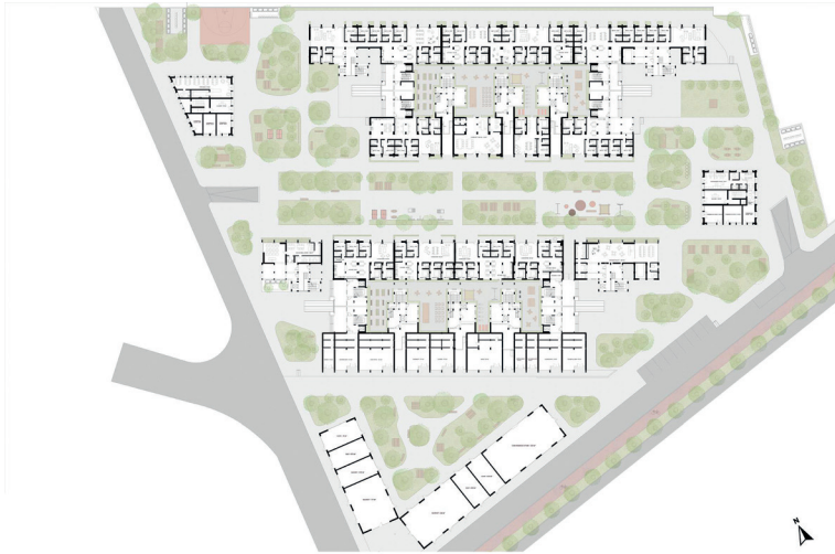
Figure 2. A balanced distribution of green spaces and activity spots throughout the plot. The west tower stands as a landmark parallel to the street while the east tower stands in axis with the new central public space completing it. A set of new shops create the south triangular piazza. Apartments show a zigzag of private and social spaces, with courtyards for collective activities (Authors: R.B. Madeira, B. Savin, A. Trsic, A.A. Zaorska, 2025).
