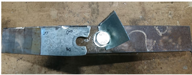
Specimen 1.2-15-w-50 Net section failure
