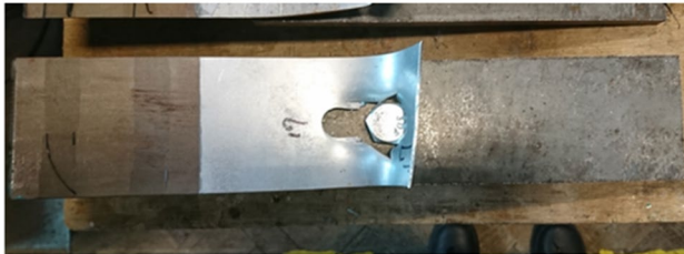
Specimen 2.0-10-wo-75 Bearing failure
