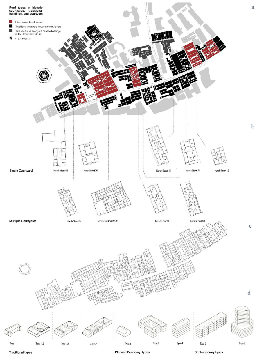
Fig. 7.32 Elaboration showing the characteristics of courtyard types and typological process in Nanshijie Street: a roof types in traditional and historic buildings; b plans of typical courtyard types; c typological plan of Nanshijie (drawn and arranged after the survey by the Cultural Relic of Guizhou in 2017, and our workshop survey); d main typological process in the whole block (drawn by Pezzetti L.A.)
