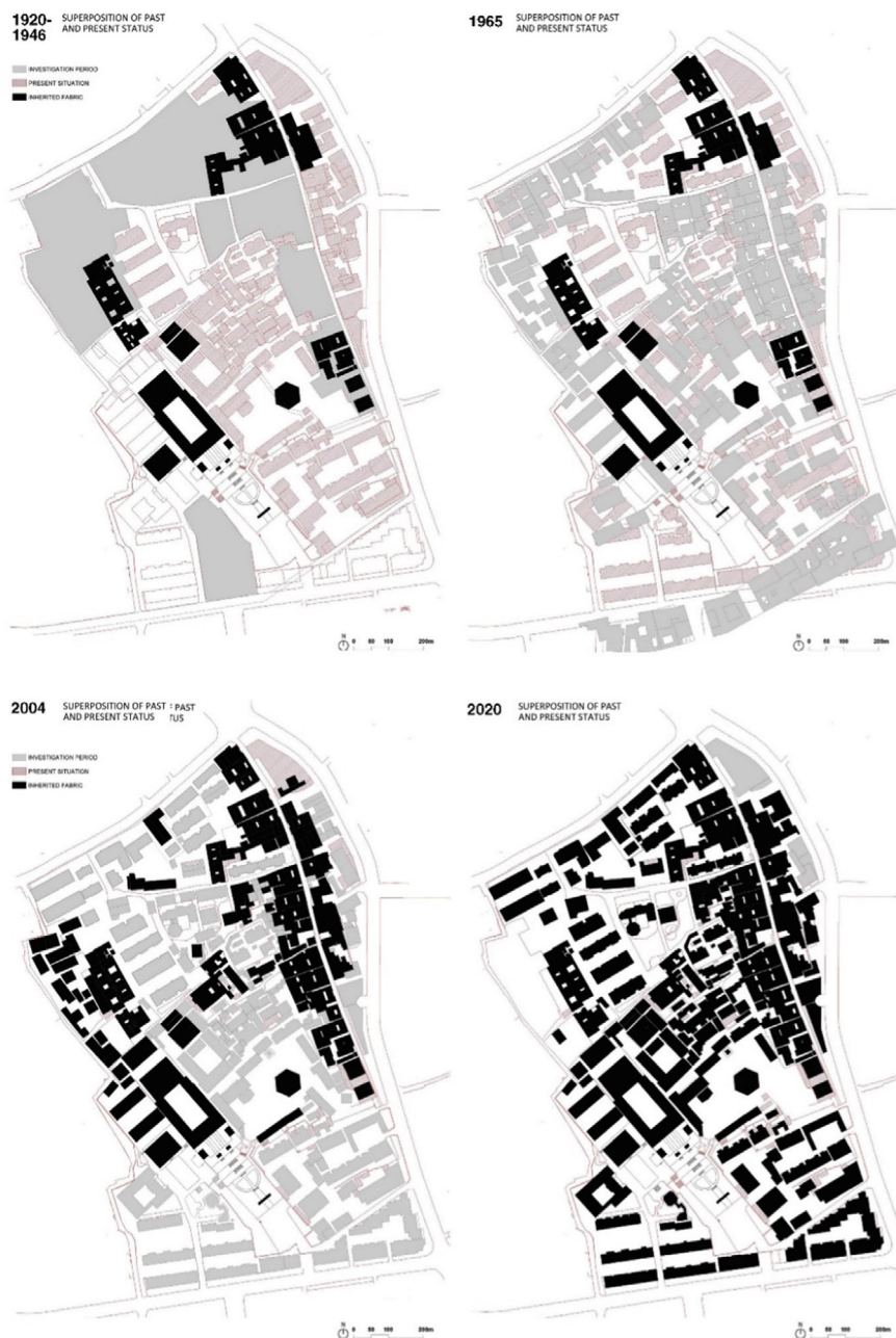
Fig. 7.20 Synchronic superposition of four morphological periods (1912–1946; 1965; 2004; 2020) analysing permanencies and transformations (in black, the previous period; in grey, the historic section; in red, the present time) (drawn by Pezzetti L.A. in the Collaborative Class)
