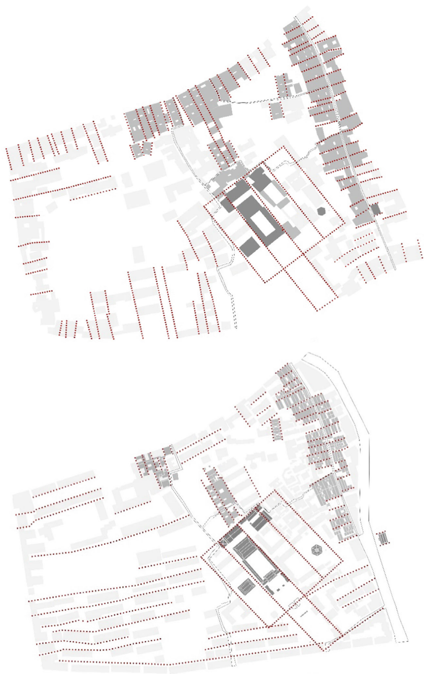
Fig. 7.29 Typo-morphological interpretative mapping of Nanshi block showing the patterns formed by the building types in 1965 (primary elements, courtyard houses and traditional dwellings) and in 2021 (primary elements, courtyard houses, traditional dwellings and modern linear building) (drawn by Pezzetti L.A.)
