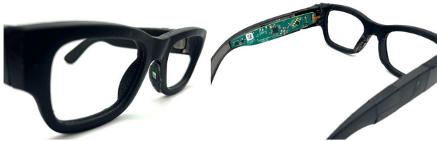
Fig. 2. Fully assembled system embedded into a standard eyewear frame. The green LED light from the PPG sensor placed on the left nose pad is clearly visible (Left). Partially disassembled view, showing the integration of the main board on the left temple and the nose pad probe on the left nose pad (Right).
