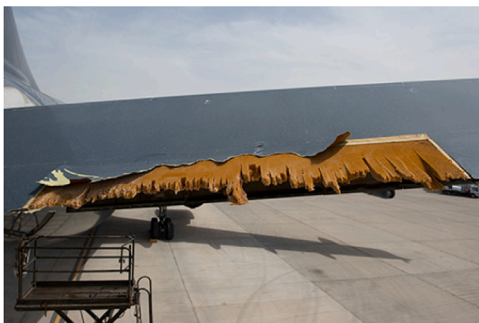
Fig. 2. View of damaged right elevator trailing edge of an A310 Polaris. Adapted from [18].
