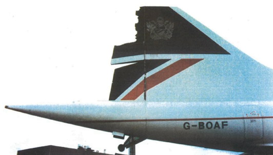
Fig. 1. Rudder failure, G-BOAF, 1989. Adapted from [10].
