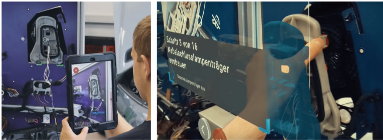
Fig. 6. Developed MAR Application for CT Scenario (4) at the Chamber of Crafts for Lower Franconia in Schweinfurt, Bavaria (Germany)
