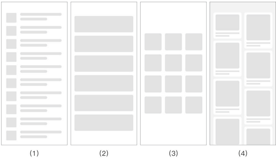
Fig. 1. The figure shows four mobile terminal information layout methods, they are (1) list layout, (2) card layout, (3) palace format layout, and (4) waterfall flow layout.
