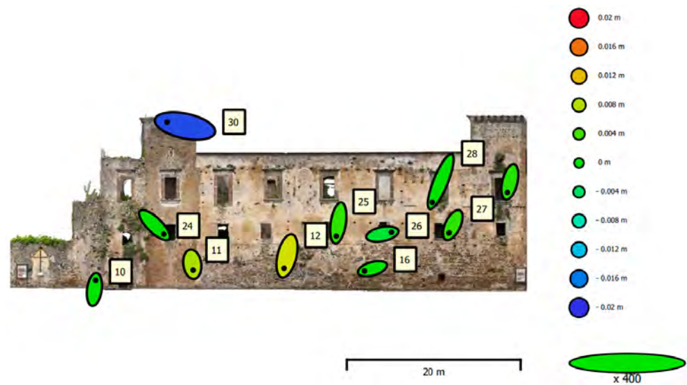
Figure 8. Position residuals represented as error ellipses based on GCP and CP positions for the analysed castle facade. Error ellipses are enlarged by a factor of 400.
