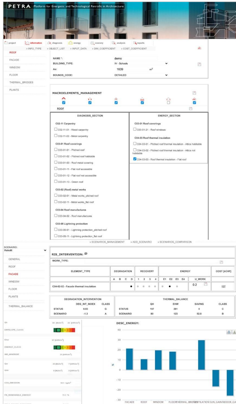
Figure 6 – PETRA tool [46]. After filling in the building information required (including heritage value, building component characteristics and thermal zones parameters), retrofit solutions can be selected and ranked according to advantages in energy, heritage protection and cost.
