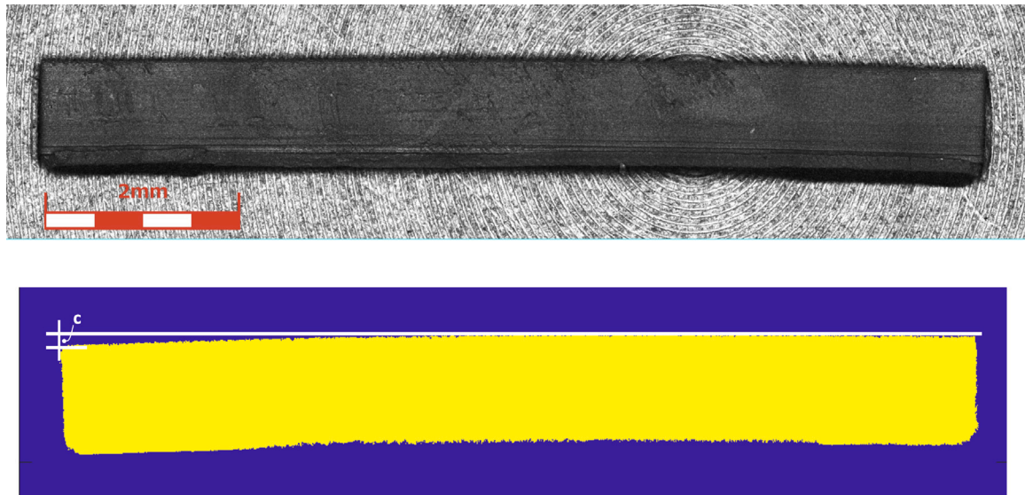
Fig. 4. Definition of the deviation from rectilinear geometry for beam samples; top panel: laser intensity image; bottom panel: top surface mask (yellow pixels) obtained through the height laser data; definition of the deviation c is reported.
