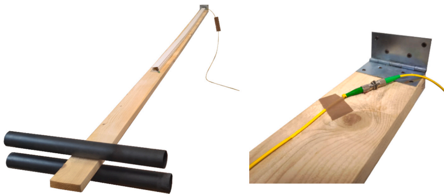
Fig. 4. Laboratory setup of the simply supported timber beam test specimen.
