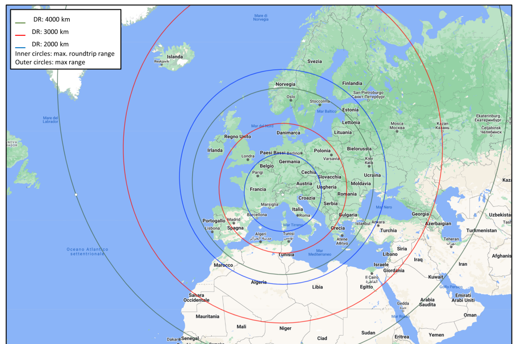
Figure 5. Design range (outer circles) and maximum range for single refueling return trips (inner circles) for aircraft with a 2000 km (blue), 3000 km (red) or 4000 km (green) design range.
