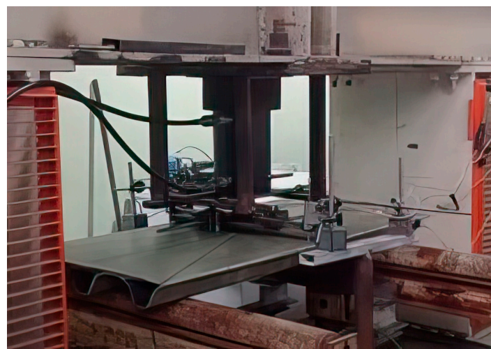
Figure 15. Testing rig for three-point bending test (Nugae panels).
