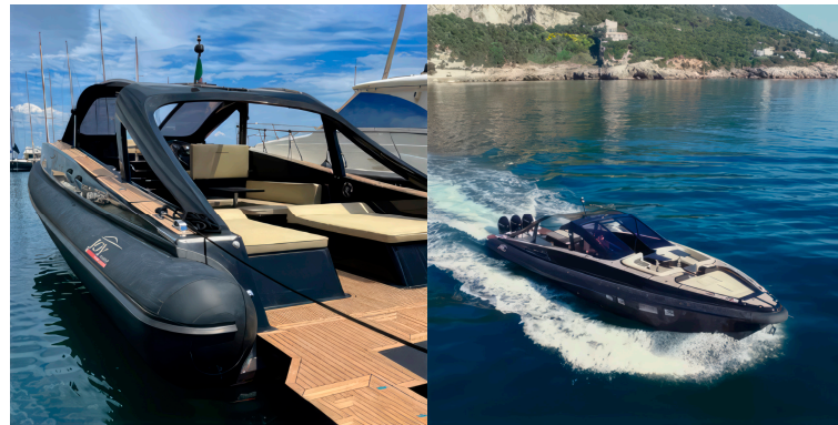
Figure 21. Three-dimensional-printed hardtop mounted on the RIB.
