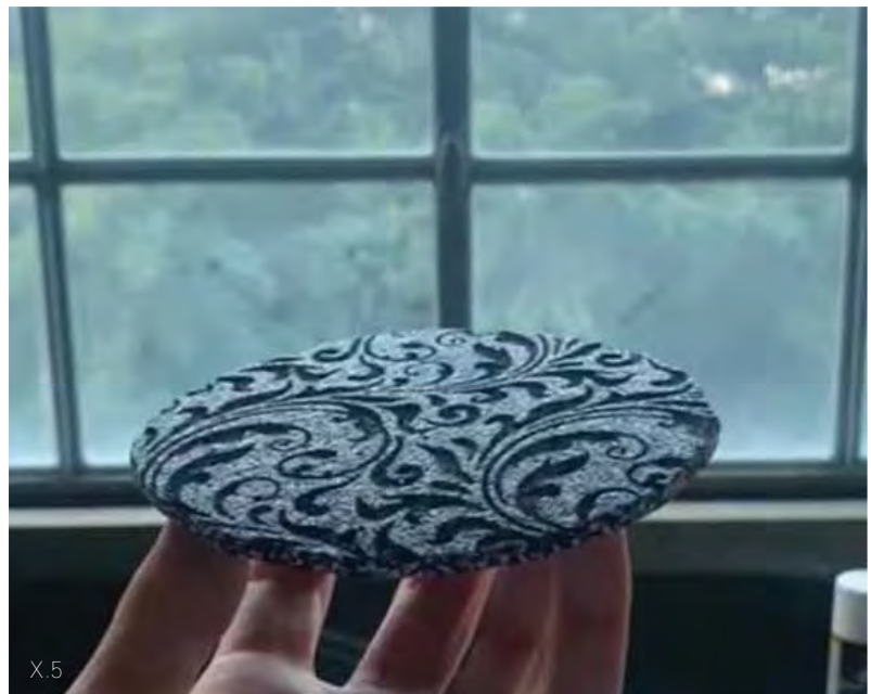
FIGURE X.5 - A study of surface decorations made by digital fabrication on recycled material from the soles of sports shoes. The aesthetics of the material change depending on exposure: when exposed to direct light, the workings on the material are barely perceptible, while against the light the texture becomes evident. Research commissioned by ESO, 2021 (Source: Ghigos)
