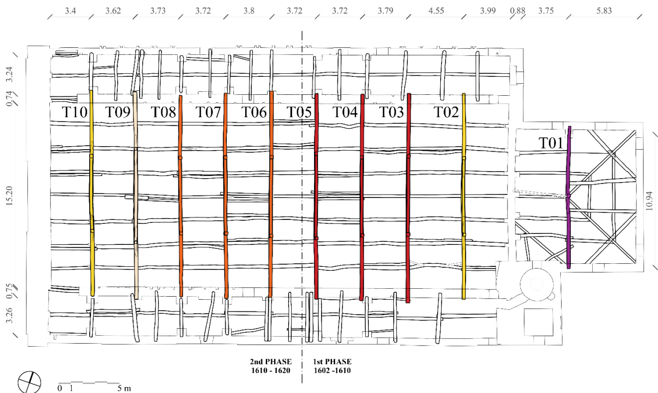
Fig. 5. Plan of the roof structure. (Geometrical survey: Courtesy of R.T.C. di Colturato & Pedrini). In purple the king post truss of the roof of the presbytery (T1); in red the Palladian trusses of the first phase in which the queen posts rest on the tie-beam (T3-T5); in orange the Palladian trusses of the second phase in which the queen posts are linked to the tie-beam with tenon-mortice joints (T6-T8); in pink the Palladian truss reworked probably in the first decades of the 19th century with queen posts detached from the tie-beam (T9); in yellow the Palladian trusses reworked in 1841 with queen posts detached from the tie-beam (T2 and T10).
