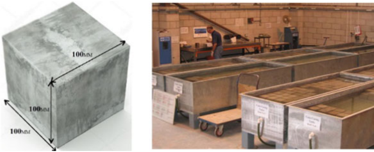
Fig. 3 Determination of water absorption of concrete specimens
