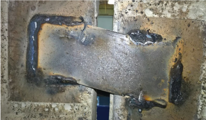
Fig. 1 Destruction of the connecting plate during shear
