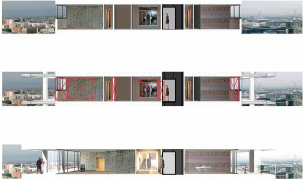
Fig. 4 - From above: existent and transformation projects. Perspective section of the project 'from the inside'. Transformation de la Tour Bois le Prêtre, Paris 17 e , Paris, France, 2011. Source: El Croquis "Lacaton & Vassal 1993 2015 - Post media horizon", 177/178. p 228.
