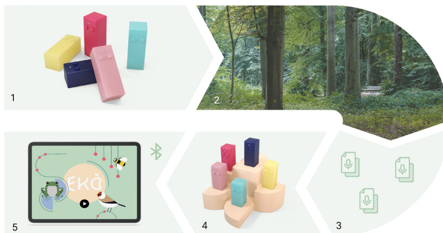
Fig. 7. The Ekō components and interaction process. Ekō recorders are used in the nature environment to look for and register nature sounds. The control base enables the transfer of the recorded sounds to the Ekō app, where they can be played and composed within audio–visual mashups.
