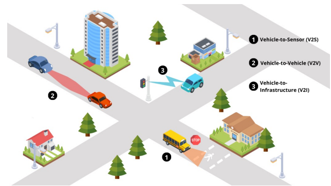
FIGURE 1. Vehicular network scenario highlighting V2S, V2V and V2I applications
