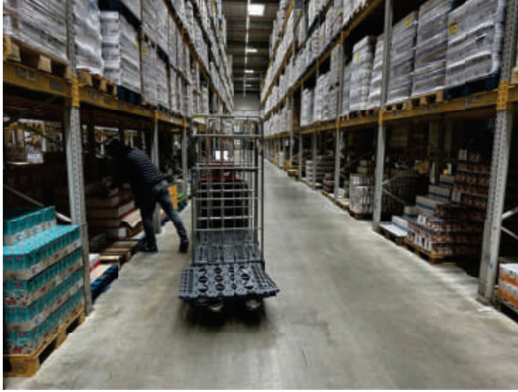
Figure 2: Picker-to-parts order picking system with vehicle support by industrial trucks.
