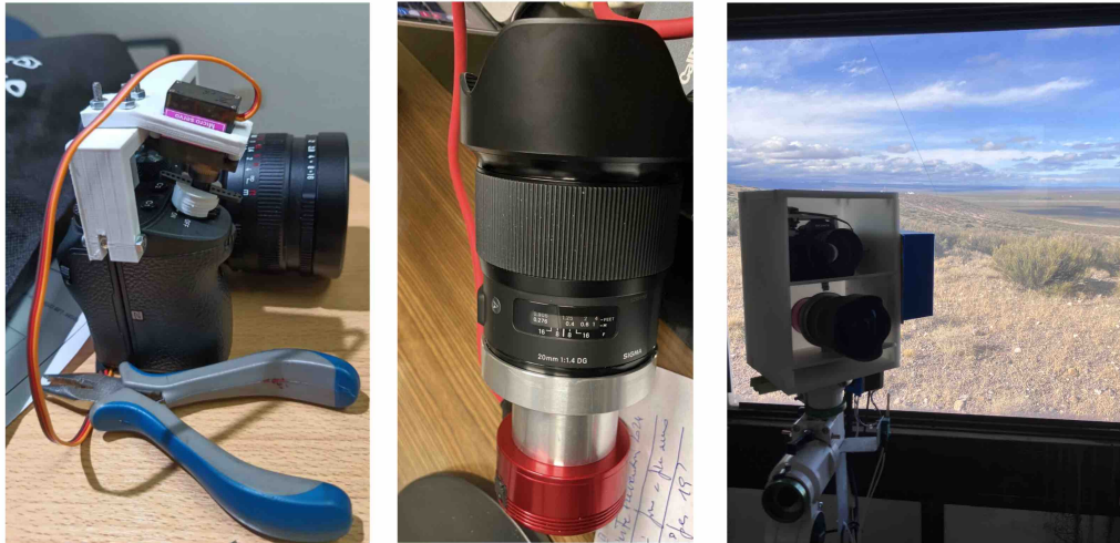
Figure 1: The new TLECAMs: Sony \alpha 7-III (left), ZWO ASI294MC (center), mounted in parking position with the field of view on the back (right).
