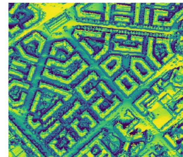
Figure 10: Lidar map relating to tree volumes. In order to reduce the inaccuracies due to the low resolution, buildings have been eliminated from the map by using a mask increased by a buffer zone of 3 meters. To reduce some defects detected at higher altitudes, interval from 1 to 20 m from the ground has been considered (the white parts of the trees refer to volumes above 20 m).
