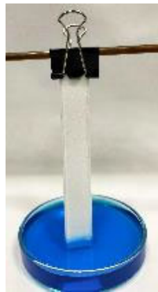
Figure 2. Setup for capillary rise tests.
