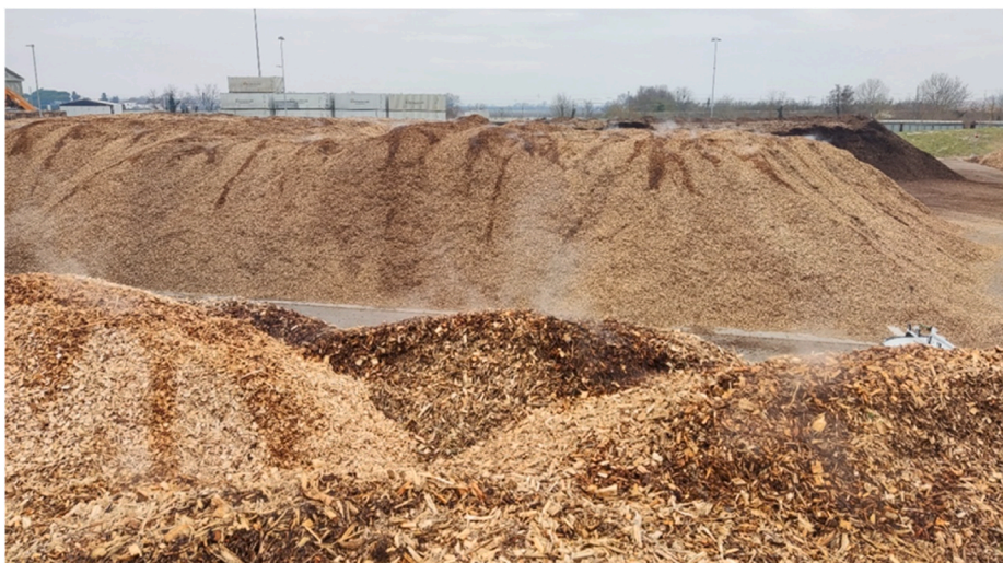
Fig. 1. Picture of a biomass heap taken in March 2022: it is possible to discern visually smoking regions from dry ones.
