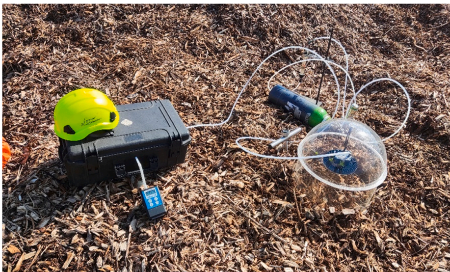
Fig. 2. Gas sampling system employed during experimental campaigns.
