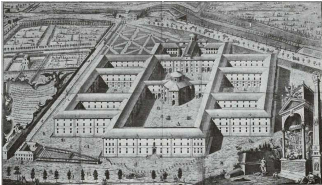
Figure 6. Perspective view of the proposed Albergo dei Poveri in Milan, by Giulio Galliori (late 18th century). This architectural rendering illustrates the ambitious plan by Giulio Galliori for a large-scale Albergo dei Poveri in Milan, designed as a centralized facility for the care, labor, and correction of marginal populations. With its symmetrical layout, separate pavilions, and central church, the project embodies the functional and disciplinary aesthetics of the Teresian and Josephine reforms. Although never completed, it strongly influenced other welfare institutions across Lombardy
