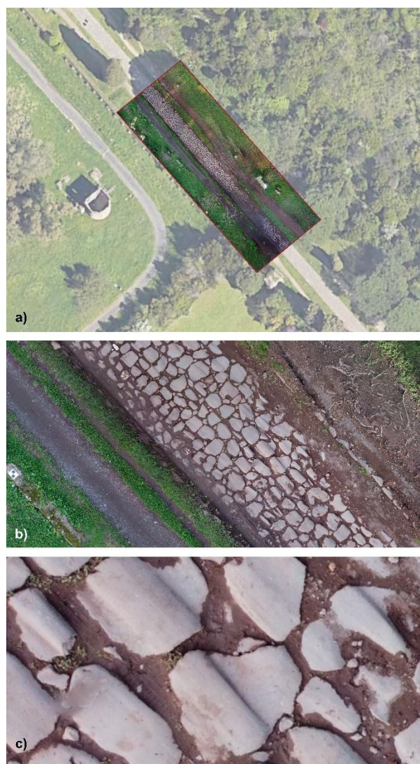
Figure 7. The Orthomosaic output obtained at different scales and resolutions (a–c) and the horizontal plane to be managed within CAD tools.
