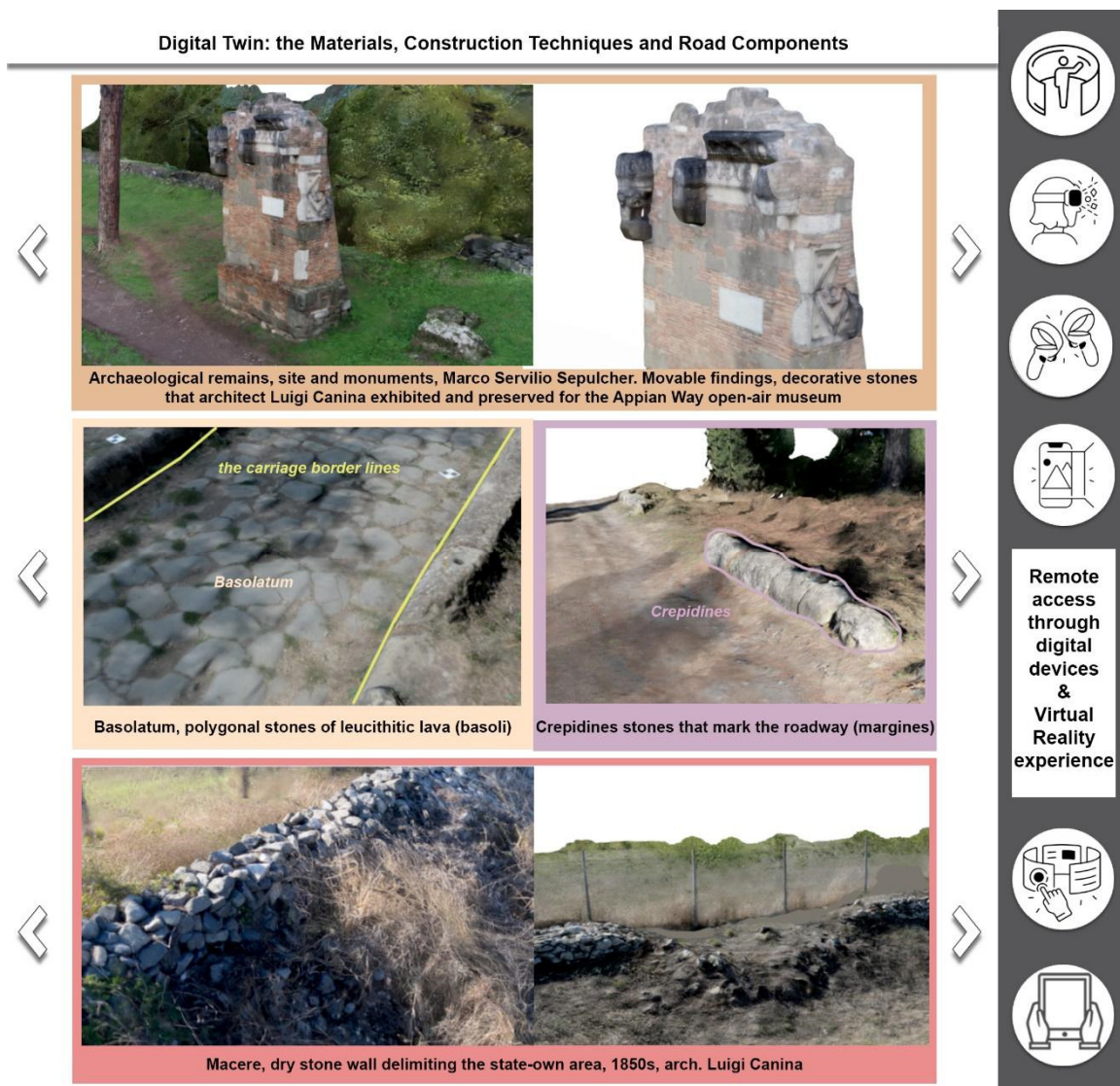
Figure 23. eXtended Reality multi-layers multi-temporal multi-scale informed models rising awareness among visitors. Visitors can read the different layers and components, understanding the material and construction techniques of the Appian Way, which is generally unknown as the Pavimentum , the Basolatum , the Crepidines , and the Macère walls.
