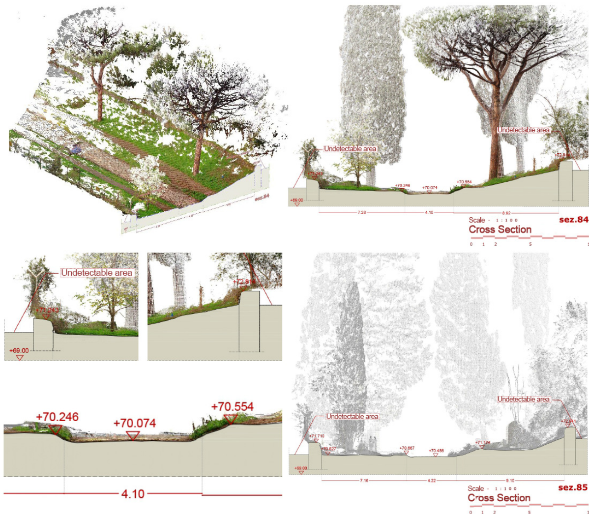
Figure 13. The Appian Way CAD Portfolio. Detail of the Transversal vertical sections 84 and 85 derived from the cloud points models (TLS, MMS and Photogrammetric models).
