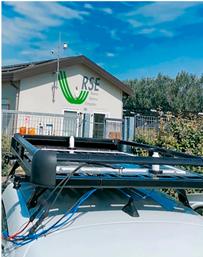
Fig. 5. "Photovoltaic roof rack" integrated on a company fleet vehicle during the measurement campaign.
