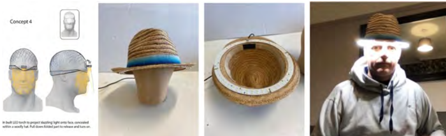
Fig. 8. The ‘halo hat’ with a ring of LED around the brim. The on-off control is a simple switch.
