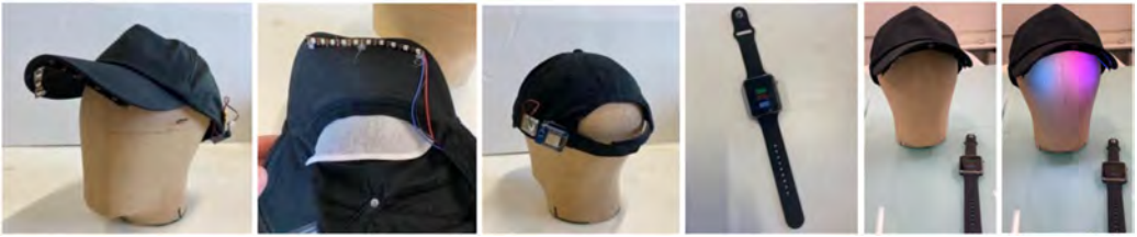
Fig. 10. The rainbow hat and the smart watch used to control it: a line of coloured led below the visor of the cap projects animated coloured lights on the face. A smart watch controls the on-off switch of the light without attracting attention.
