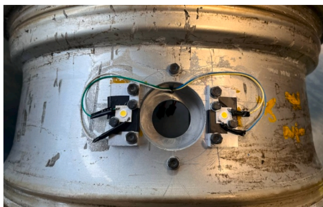
Fig. 4. Lightning system and camera support assembled on the rim.
