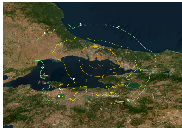
Figure 6. The intensity distribution in Istanbul Damage Modeling and Estimates: The intensity based empirical vulnerability relationships developed by Lagomarsino and Giovinazzi (2006) are used to estimate RC damage grades (D3-D5) (see also Figure 7).
