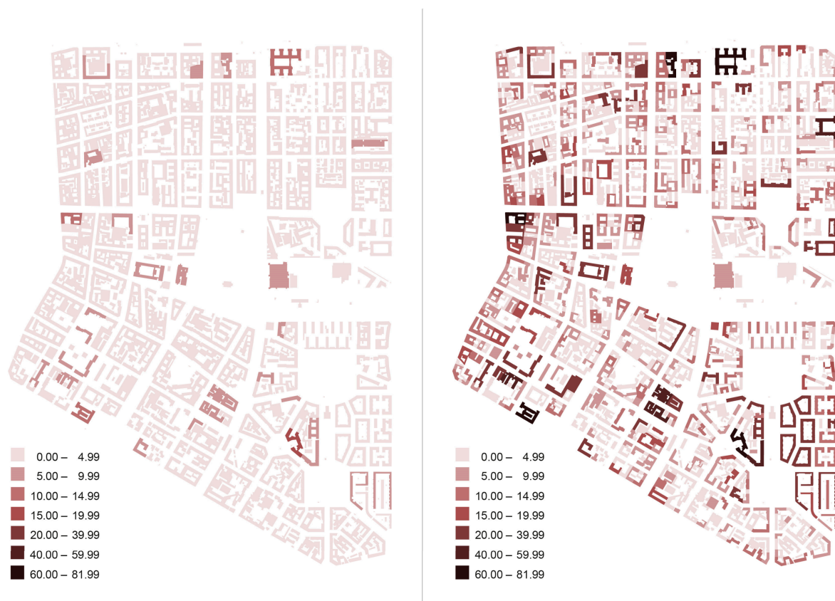
Figure 7. Spatial distribution of concrete ( left ) and masonry ( right ) referred to the boundary of analysis (thousands of cubic meters).
