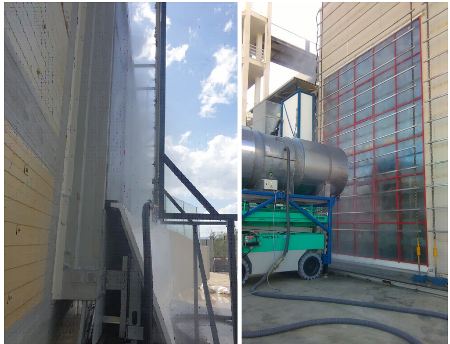
Fig. 25 - Simulazione bomba d'acqua in assenza e presenza di vento / Water bomb simulation in the absence and presence of wind (Source: Authors' elaboration).
