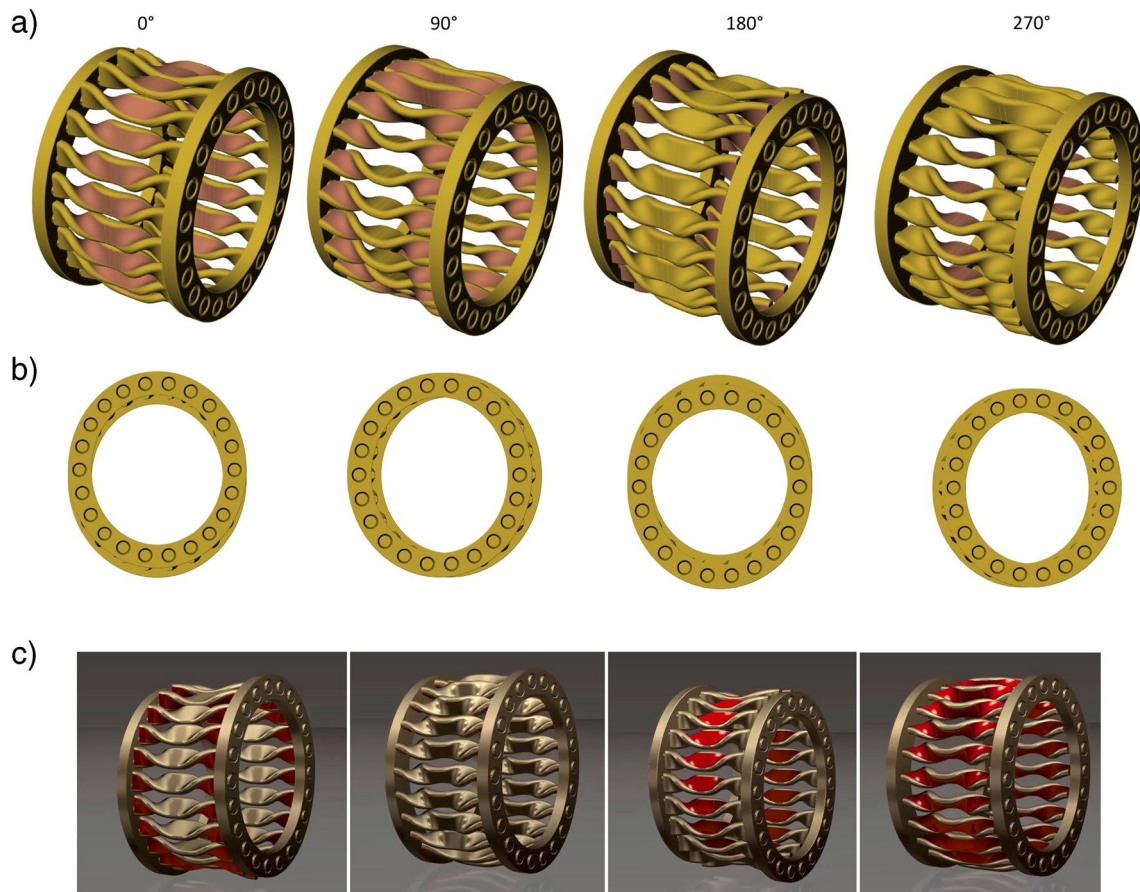
Fig. 9 The mechanism that allows mimicking the snake ventral scale slithering. a Isometric views of the jewel at four stages of the rotation (0°, 90°, 180°, and 270°). b Lateral views of the entire jewel at the same four stages. It is possible to notice the translation of the two
