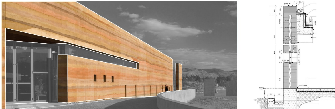
Figure 6. Rammed earth façade and detail - Nk'Mip Desert Cultural Centre by Dialog
