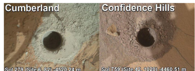
Fig. 5. Two examples of images of drill holes performed by NASA's Curiosity Rover respectively on Yellowknife Bay (Cumberland location, left image) and Confidence Hills (right image) in Gale Crater on Mars. The diameter of the holes is 1.6 cm. Images have been taken by the rover's Mars Hand Lens Imager (MAHLI) camera. From https://photojournal.jpl.nasa.gov/catalog/PIA21254 . Credits NASA/JPL-Caltech/MSSS/UA.
