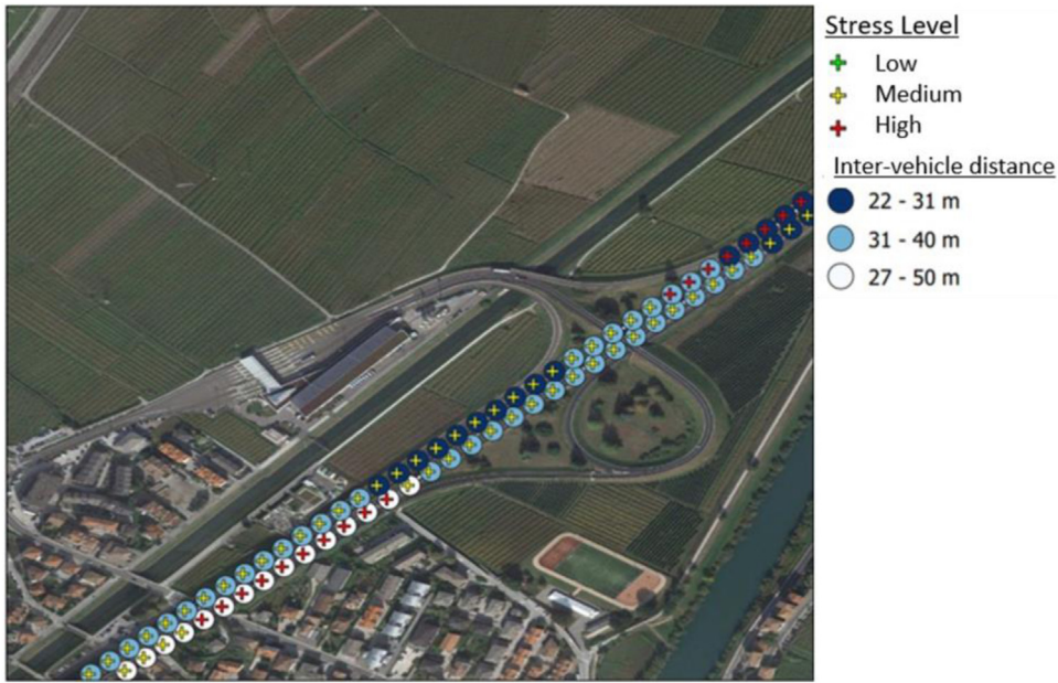
Fig. 18. Follower vehicle, high stress level nearby a sample motorway junction.
