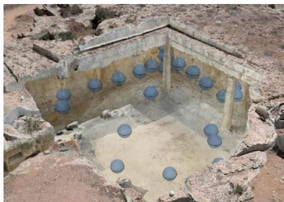
Figure 5. 360 images block geometry - XPhase Pro X2.
