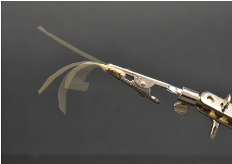
Figure 1. Chitosan sustainable actuator (Den Teuling et al. , 2024). Photo Credits from the authors of the projects.
