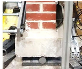
d) Roller under wall specimen
