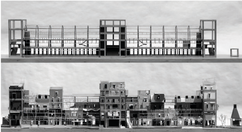
Figure 5. L'ecomostro addomesticato. Existing reinforced concrete structure (top) and integration of new volumes from secondary materials (bottom) [Source: Studio Albori].
