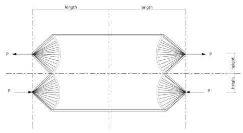
Fig. 2a. Cox's optimal beam for bending.
