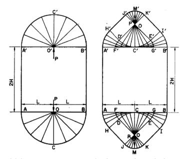
Fig. 4a. Optimal disks carrying two concentrated and opposite forces; the design is to lie beyond the region ABA'B'.
