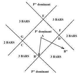
FIG. 5. Truss type as a function of the alternative loading.
