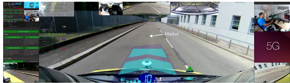
Figure 5. Snapshot of visual feedback at the control station. Displaying left, front, cabin, rear, ground, right, and control-station footage.
